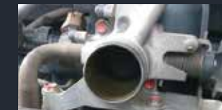
BEFORE (Throttle body condition after 60,000 km)
